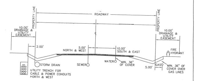
1. DIMENSIONS FOR LOCATION OF UTILITIES ARE THE SAME WHETHER THE ROAD ARE ASPHALT WITH CURBS, GUTTERS, AND SIDEWALKS; ASPHALT WITHOUT CURBS, GUTTERS, OR SIDEWALKS.
